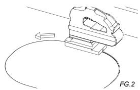
2. Cut out the counter -The cutting tools required will depend on the surface to be cut. *FG.2*
