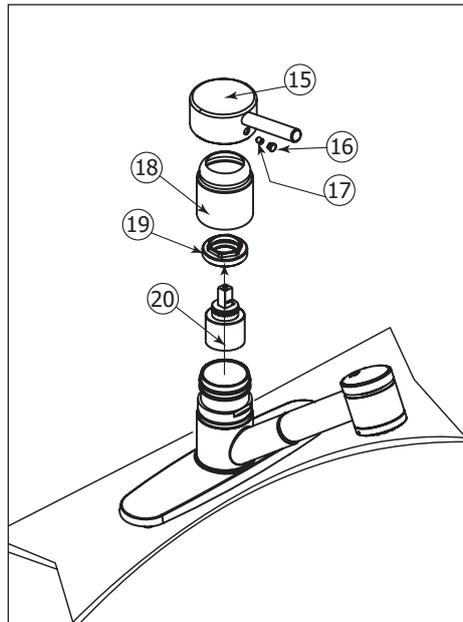
To replace the cartridge, start by shutting off water supply lines and then turning on the water to drain the faucet. To replace the cartridge (20), pull out the handle (15) by removing the cap (16) and the setscrew (17) first. Afterwards, remove the dome cap (18) and the retainer ring (19). Replace with new cartridge and reassemble by reversing steps.
