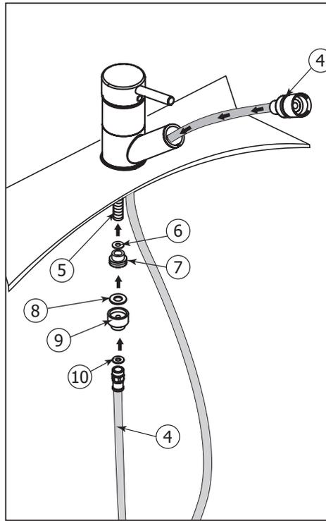
Ensure the fitting (7) and its washer (6) are well tightened onto the center tie-down (5). Afterwards, firmly screw the adapter piece (9) and its washer (8) onto the other end of the fitting (7). Finally, slide the handshower hose (3/8" male) (4) into the spout base and screw it onto the adapter (9).
