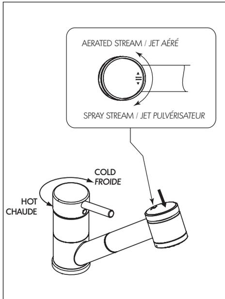
To turn on water, lift the lever handle up, increasing the flow gradually. Turn handle to the left to increase hot water flow and to the right for colder water. This pull-out spray faucet is equipped with two types of water stream modes: aerated and spray. The default mode is aerated. To switch to spray stream mode, press down the top button on the spray head. To keep it in spray mode, turn the button clockwise once pressed down as shown. Turn button counterclockwise to return to aerated mode.
