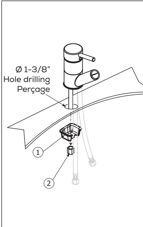
**!** We recommend drilling a 1- 3/8" diameter hole for the insertion of the faucet
