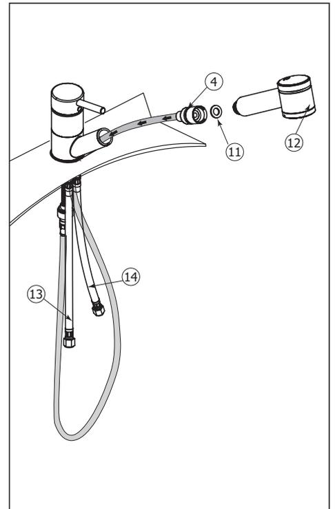
After installing the faucet, connect the hot (RED) and cold (BLUE) (13) (14) 3/8" flexible hose inlets to the water supply lines. Before connecting the spout, turn on hot and cold water in order to flush residue and impurities. After this step, connect the spout (12) and washer (11) to the hose (4) (See Fig.4).
